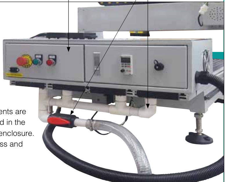
The rear view of the Techno HD II 21 x 36 Tabletop CNC Router is showing the electronics enclosure and vacuum connections
